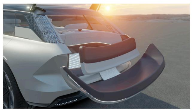
While the interior is designed for only four people, the rear split gate can be turned into a rear seat, with a seat back that folds out from the cargo area and the seat bottom formed from the tailgate panel, though this presumably is only for when the Star is parked.
